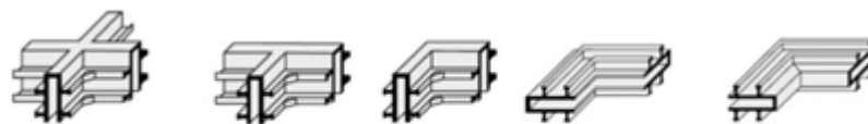
Cross piece vertical T-piece vertical L-piece vertical L cross piece flat L-piece flat, cover slab inside
