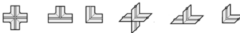
Cross piece flat T-piece flat L-piece flat Cross piece vertical T-piece vertical L-piece vertical
