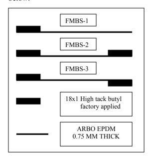
Available in 0.75 mm thickness, 25 metre length rolls.
