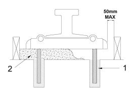
Example of Conbextra EP grout to machinery baseplate:
