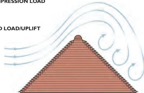
InSkew has been designed to resist both the sliding and compression loads of the roof covering while also counteracting the tensile loads caused by wind uplift.
