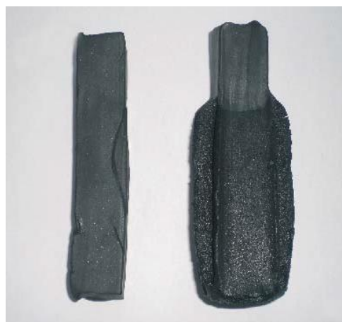
KÖSTER Quellband before and after reaction
