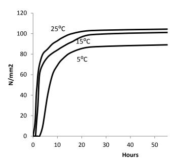
Note: The performance of Nitomortar PE winter grade at 5°C is similar to that of the standard grade at 20°C.
