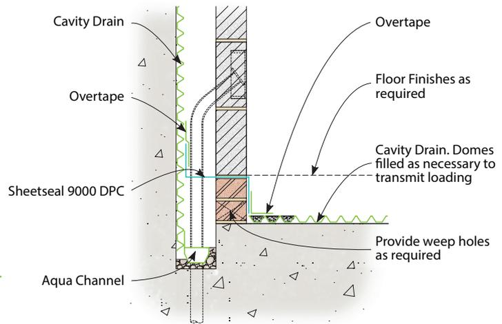
Wall Floor Junction with Masonry Lining Wall
