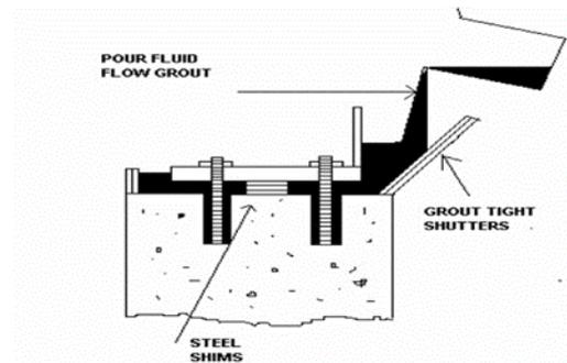
Set grout should be chamfered to ensure that unrestrained shrinkage cracking does not occur.
