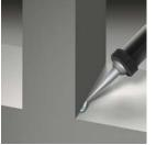
Figure 3: Apply a 10 mm diameter bead of SP525 to bottom corners of the window opening to match joint depth of tape
