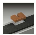
Figure 6: To accommodate setting blocks, notch out tape
