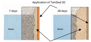
Crystals growing into the concrete
