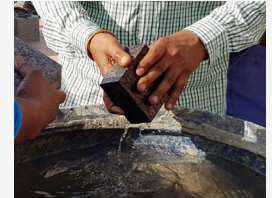
Clean area and underside of paving units
