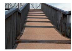
Preformed Surface Dressing is an exceptionally versatile, ready-to use, hard wearing skid resistant surface for pedestrian trafficked areas. It comprises of a high performance polymer modified bituminous binder and a layer of skid resistant calcined bauxite chippings, strengthened by an integral mesh. Preformed Surface Dressing can be used on most surfaces, including wood, concrete, asphalt and steel.
