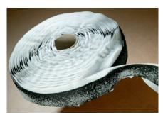
Gripstrip is an anti-skid, self-adhesive, overbanding joint and crack sealing tape. **Gripstrip** consists of an extruded bituminous compound modified with elastomers and fast bonding resins. It is extremely safe and convenient to use as it does not require any heating or mixing.
