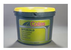
Bitukold is a cold hand applied, thixotropic bitumen emulsion designed for sealing vertical joints. On small patches, Bitukold can also be used as a tack coat, thereby saving on the need to use a separate tack coat emulsion. Bitukold is mainly used for the protection of new joints in freshly laid asphalt or macadam.
