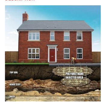
GeoTek LV is a low viscosity, single shot polyurethane based on MDI in combination with polyether polyols and an amine based catalyst. The system only reacts when it comes into contact with water, forming a rigid polyurethane foam.
