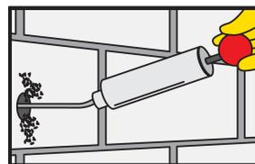
The drill hole must be cleaned with a blow pump or by compressed air (Re-bar application), starting from the bottom of the hole. (at least 2x) Important: use oil-free compressors.
