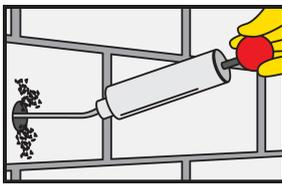
The drill hole must be cleaned with a blow pump or by compressed air (Re-bar application), starting from the bottom of the hole. (at least 2X)
