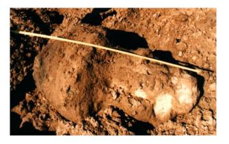
GeoTek AC is a two-component ultra-low viscosity hydrophilic acrylic grout, which when set forms a resilient gel. Adjusting the amount of accelerator varies the gel time to enable greater control on site.
