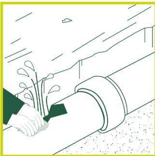
Apply the paste to the damaged area or leak and hold firmly in position without movement until set.
