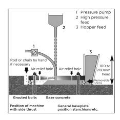
The diagram illustrates typical methods of placing **webercem advanced precision grout SP**.
